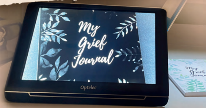
Above: "The Ruby" by Optelec. It is an electronic magnifier and is available through the CNIB, Vision Rehabilitation Division.
